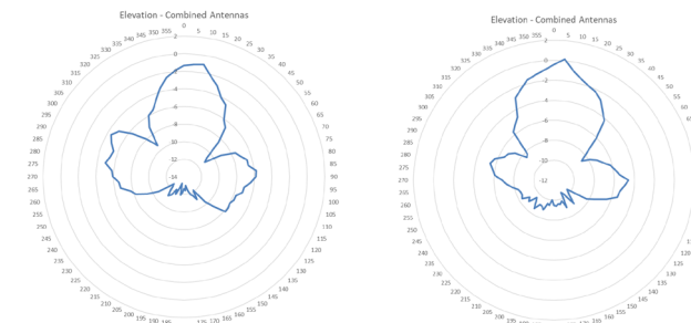
RG-AP680(CD) 2.4GHz (Left) and 5GHz (Right) Elevation Antenna Patterns
