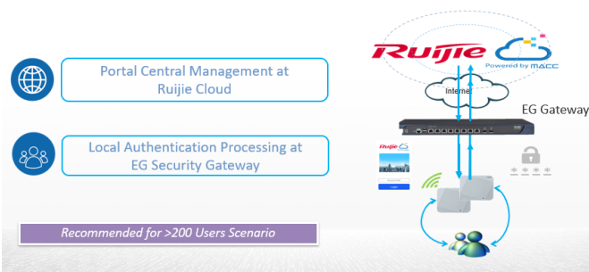
Ruijie EG's Authentication Offload and Acceleration
